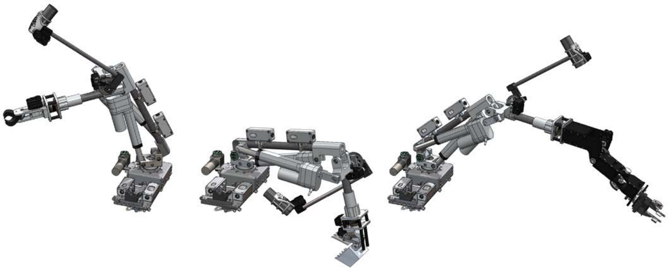
Figure 18. The robotic arm. Designed, built and included on the 2011 OSU Mars Rover. (left) setup for the Astronaut Assistance task and reaching towards the rear of the rover (center) Setup for the Soil Sample Return task reaching towards the ground to acquire a sample. The arms camera is positioned to view the sample as it is captured by the scoop. (right) setup for the Equipment Servicing task
