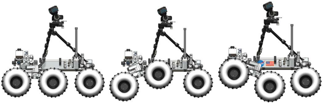
Figure 8. Range of motion of the front rockers (left) neutral position (center) counter-clockwise rotation limit (right) clockwise rotation limit
