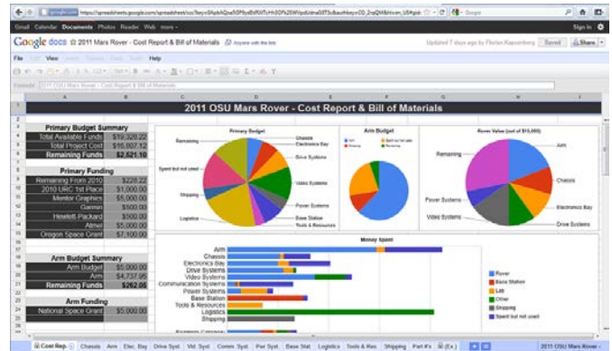
Figure 51. The summary report page of the Bill of Materials (BoM) for the rover project. Summarized here are current spending allocations compared against available funds categorized into subsystem spending and useful versus waste expense. The BoM is a Google document which is easily accessible by any team member and is updated in real time.
