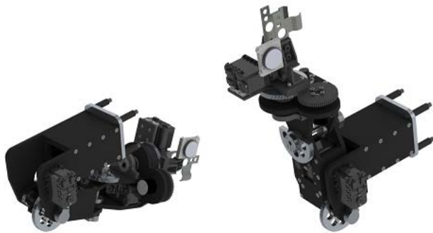
Figure 28. (left) Equipment servicing end effector shown in stowing configuration (right) showing pitch upward range of motion
