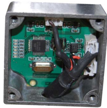
Figure 32. Servo controller PCB shown in water proof housing
