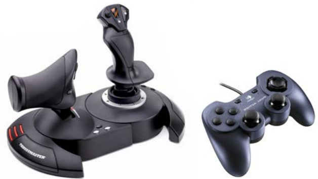
Figure 43. (right) controller used to drive the Rover and aim and zoom the main camera (left) controller used to operate the arm
