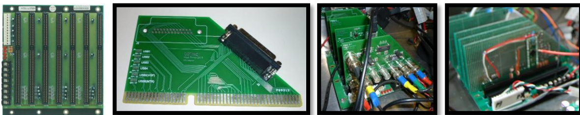
Figure 28. A 7-slot ISA backplane (first picture) allows the electrical systems to be modular. An input/output card with 29-pin connector (second picture) interfaces the electrical systems installed in the backplane with the rest of the rover (third picture). The nature of the backplane allows the cards to be inserted in any slot, and does not permit them to be inserted backwards. Boards can quickly be removed for troubleshooting, or replaced if necessary. It also allows for easy prototyping by using ISA-style protoboards (fourth picture).
