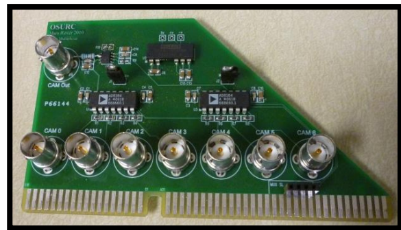
Figure 32. The Video multiplexer which mates to the rover's backplane. The upper BNC connector is the output; all other BNCs are possible input channels.
