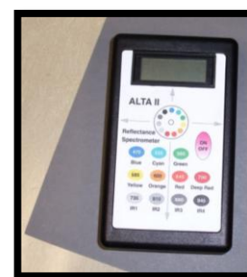
Figure 45. Reflectance spectrometer used to investigate the presence of cyanobacteria in the soil.
