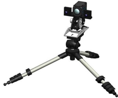
Figure 20. A camera tripod was used to mount the camera systems to the chassis. This allowed the cameras to be placed in a number of different positions over the rover depending on the task at hand.
