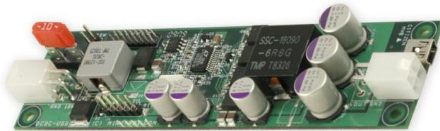
Figure 25. Automotive DC-DC converter. Output is programmable via USB.
