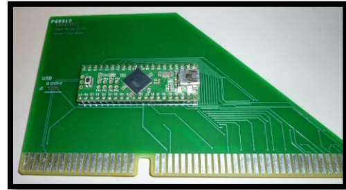
Figure 33. The Motor control card which mates to the rover's backplane. This card is responsible for interpreting driving commands and converting them to individual motor speed commands.
