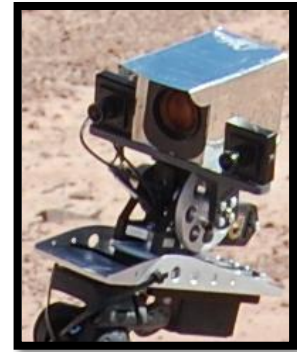
Figure 29. Primary camera atop the pan-tilt assembly. The two smaller cameras are meant for a stereoscopic viewing interface that was never fully developed.
