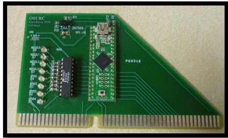
Figure 30. Video, GPS, Pan-tilt (VGP) card which mates to rover's backplane.
