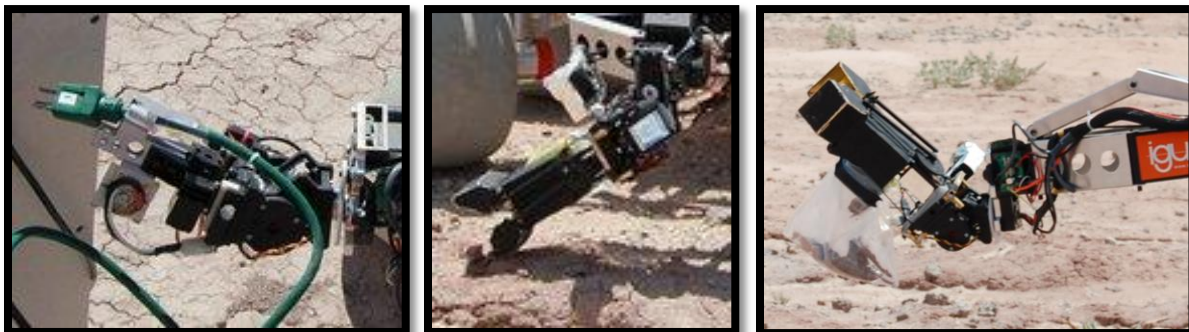
Figure 15. Two types of detachable end effectors: a gripper with vibrating motor to overcome the force required to insert the plug, and a double bucket scoop with sample bag, allowing operator to excavate large soil samples in multiple passes.
