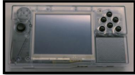
Figure 38. The Oregon State Wireless Active Learning Device (OSWALD). This small, light-weight device is the onboard computer.
