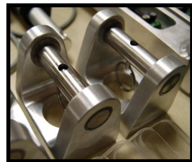
Figure 11. Interchangeable aluminum bogie hinge brackets with Nylon bushings, stainless steel axle and quick-release locking pin
